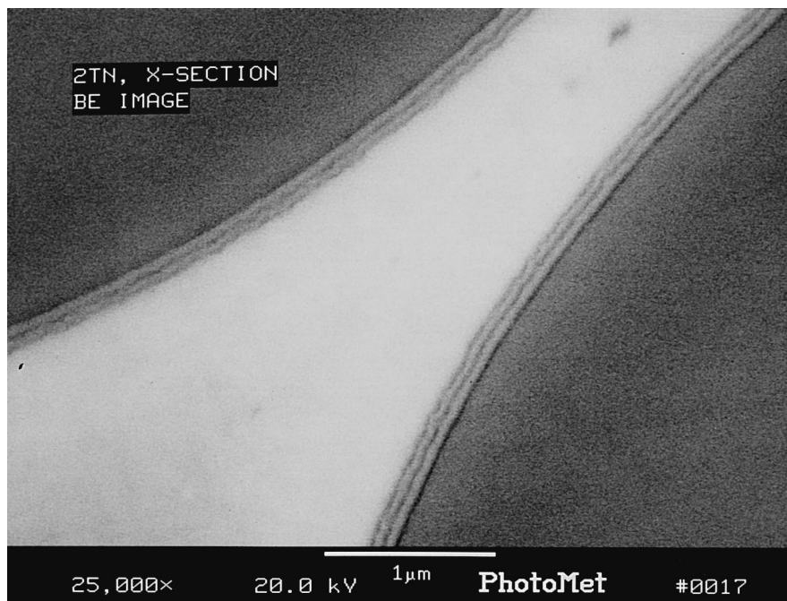
Fig. 2. Back-scattered electron image of multilayer SiC fiber coating on Hi-Nicalon fibers. SiC layers are \approx 100 nm thick and interrupted pyrolytic carbon layers are \approx 20 nm.
